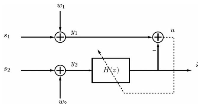
Figure 1. Block diagram displaying the adaptive filtering used to reduce wind noise in the study hearing aid.
